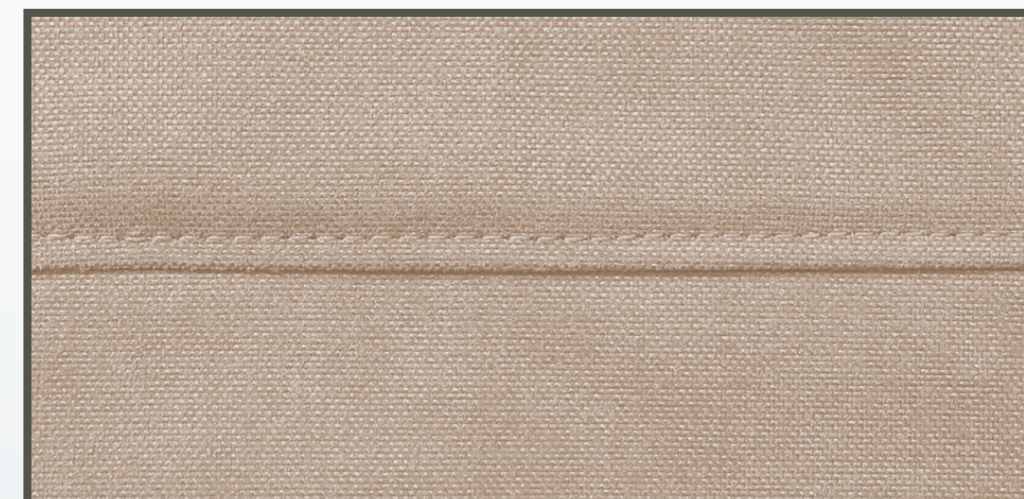
2 French Seam/ Single Needle
